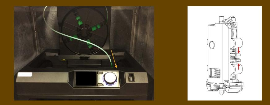
If you are loading the MakerBot with filament and cannot get the MakerBot to extrude your new colour, try pinching the black tabs on the right side of the extruder that you pressed to remove the filament.
